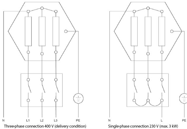
**ATTENTION, IMPORTANT: DO NOT FORGET TO CONNECT THE PROTECTIVE CONDUCTOR!**
