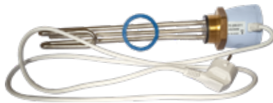
Compact heating element: 2 kW, 230 V, 6/4", single-phase
